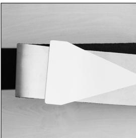
Remove the skin from the ski with jig. Replace the protective foil on nose section on the skin.
