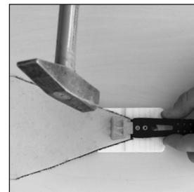
Remove the protective foil approx. 5 cm from the skin. Place the skin with the adhesive side up in the longitudinal direction on the wood panel. Pound the teeth of the Elastic Strap with a hammer straight through the skin.
