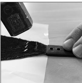
Replace the protective foil on the skin and turn it over. Pound the tips on the skin side flat with a hammer in the direction of the end of the skin, so they are at a slight angle.
